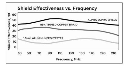
Figure 2. Foil-braid shielding yields the best shielding effectiveness
