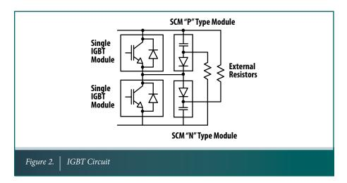
For the external resistors, thick film SMD resistors such as Bourns® Models CRM2512, CRM 2010, CRM1206, and CRM0805 have good surge capability and are available with power ratings up to 2 W. Thick film non-inductive resistors are available up to 35 W including Bourns® Models PWR163 and PWR263 in DPAK packages and Bourns® Models PWR220T and PWR221T in TO-220 packages.
