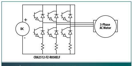
Figure 3. | Customer Solution with Bourns® Model CRA2512 Current Sense Resistors
