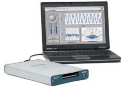
FIG 5 USB DAQ adds data acquisition to any computer with a USB port.
