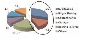
ultimately lead to motor failure and they are responsible for approximately 14% of all motor failures, while 30% are due to overloading. A motor failure is a more troubling situation, because in addition to an uncontrolled hazardous stop, it also brings with it costly downtime and repair.
